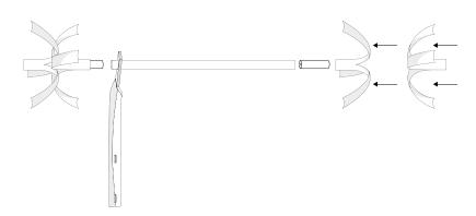
8 For ease of installation of the last shaft, load the spurs on to the shaft before connecting to the rest of the run. Fit a second locking collar up against the last support. When the last shaft is assembled and in place, tighten both locking collars and insert the last end cap.
